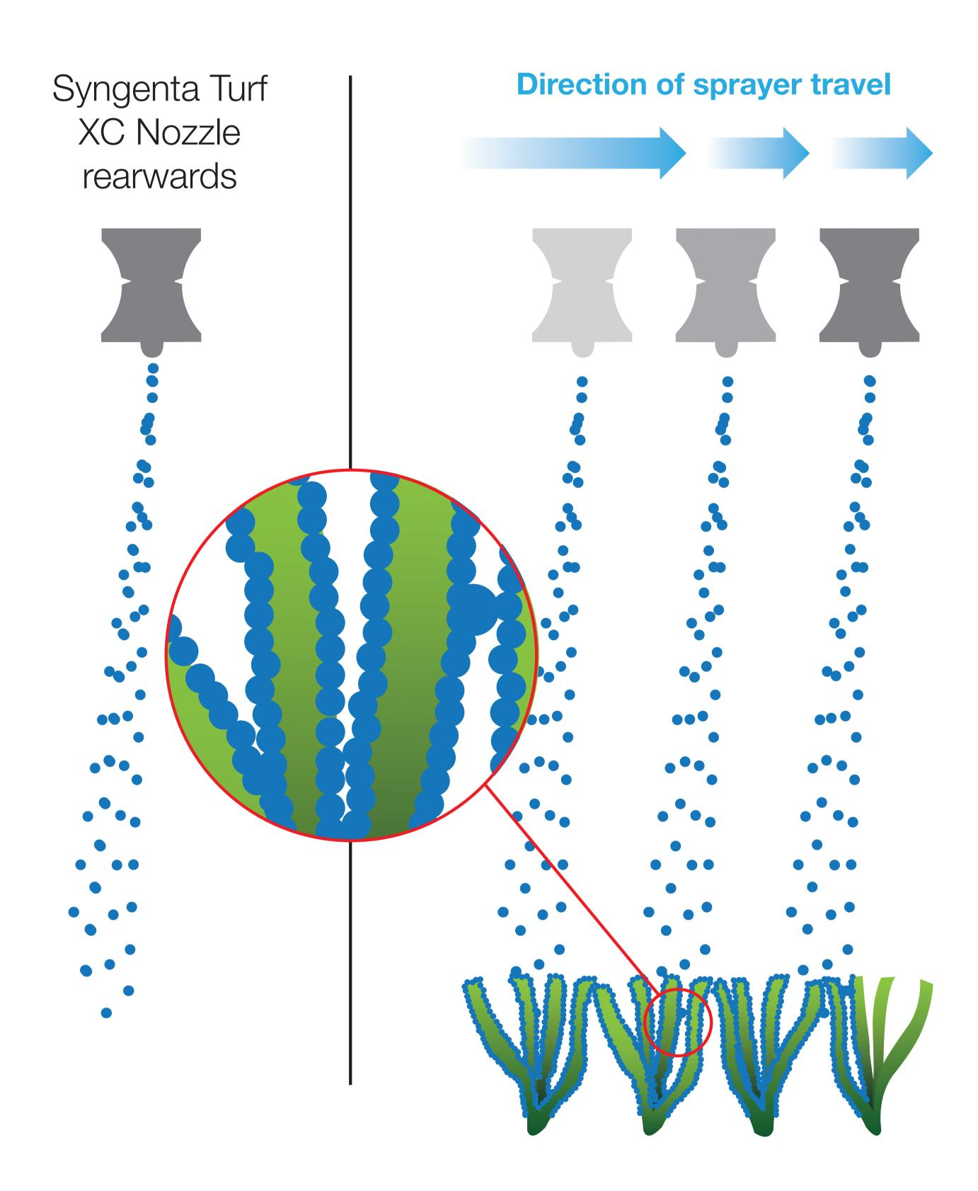
With the forward movement of the sprayer, droplets that are discharged vertically mainly hit one side of the target leaf
