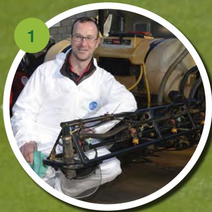
Andrew has checked the water volume marks of the sprayer tank are accurate for the amount being filled. The sprayer is always parked on the same level area for filling. Best practice is to fit a flow meter on the water filling hose, to check exactly how much is going into the tank.
