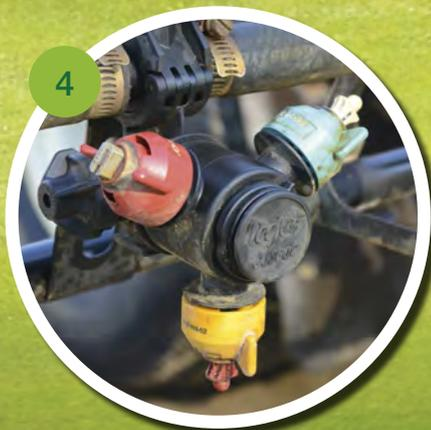
Nozzle selection is a critical part of accurate application, delivering the appropriate water volume at the required speed to hit the intended target. Andrew typically uses a water volume of 200 l/ha for foliar applied products, such as Primo Maxx or Instrata fungicide, whilst soil uptake nutrients would be applied at up to 600 l/ha to penetrate through the sward.
