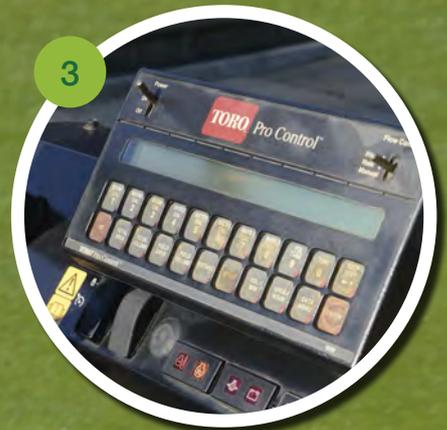
Auto-rate controllers that adjust application rate to forward speed have helped immensely with improving spray accuracy. Checking they are functioning correctly is an important element of the maintenance and calibration regime.
