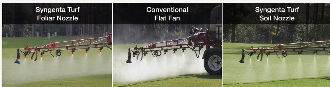
As the final point of delivery, the choice of nozzle ultimately dictates spray coverage on the leaf and, most importantly, spray retention on the intended target. Syngenta Turf Nozzles have been specifically designed to improve application techniques in turf and to enhance results that can be achieved with Syngenta Turf products. Syngenta Turf Nozzles simply fit into the existing bayonet housing on virtually all modern turf sprayers.
