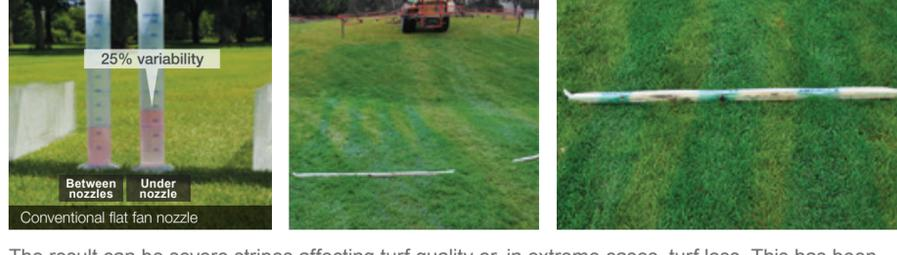
The result can be severe stripes affecting turf quality or, in extreme cases, turf loss. This has been demonstrated with spray pattern indicator above.
