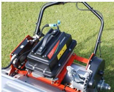
Some modern pedestrian mowers have movable engines or battery packs, which allows the Greenkeeper to change the forward weight bias of the mower to suit both growing conditions and the time of year to get the optimum results. This combined with good roller selection can greatly change the performance of the mower & the green.
