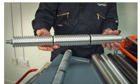
This can be alleviated somewhat by the use of a sectional roller, allowing the inside section to rotate slower than the other two during the clean up pass.
