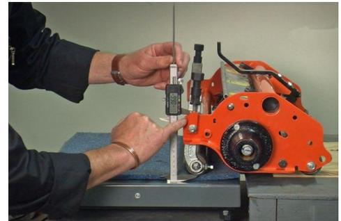
Taking a fixed datum point helps demonstrate the differences created by changing the front roller
