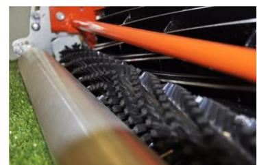
Cutting unit fitted with bi-directional brush
