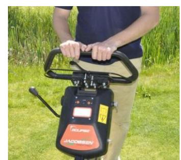
The correct method of controlling a pedestrian mower is to hold the side of the handles and “carry the handles”, keeping the handles in the middle of their mounting slots. This allows the machine to float over all the minor undulations of the green, giving a better, tighter finish to the green.
