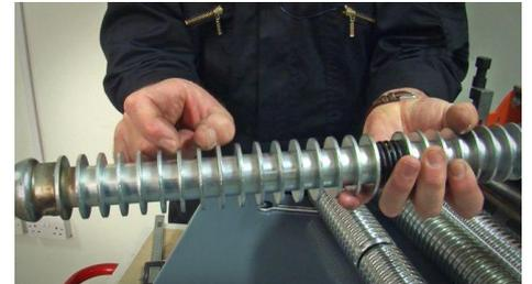
The downside to grooved rollers is surface marking and the stress affect on the grass plant when the units turn during perimeter cuts. Most modern greens triples now have steering heads to reduce side loads, but these loads are not completely removed and fitting an aggressive front roller can cause unforeseen problems in soft ground conditions or during the winter months, especially when grass growth does not keep up with the wear and tear caused by grooved rollers.
